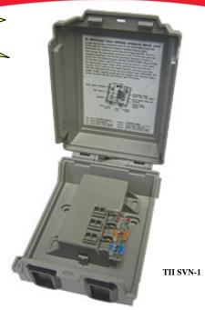
The TII Switchable Voice NID (SVN) contains a microprocessor controlled circuit that provides seamless switching from Telco service to digital phone service. The second ringing voltage appearance on the digital phone service initiates the switch over. The TII SVN utilizes gel-sealed insulation displacement terminations that provide reliable all weather connectivity.
